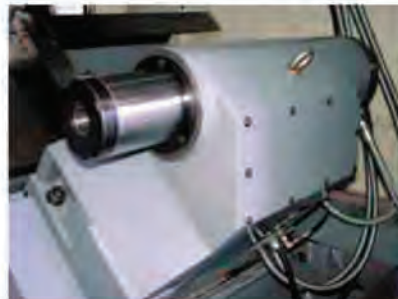
Tailstock for larger models with rotary quill.
