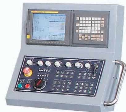
Horizontal traversable control pendant for convenient operation
